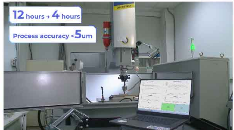
航太用AI優化放電加工設備(圖二：航太用AI優化放電加工設備 (Advanced Machining for Aerospace Applications based on AI Technology)) (Advanced Machining for Aerospace Applications based on AI Technology).
